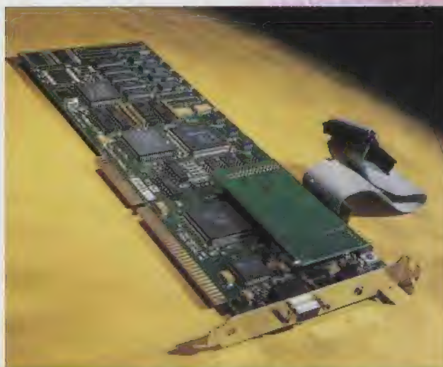
The ReelMagic board gives PCs the facility to playback MPEG 1 CDs. Like the CD 32 , it is powered by a version of the C-Cube CL450 chip
